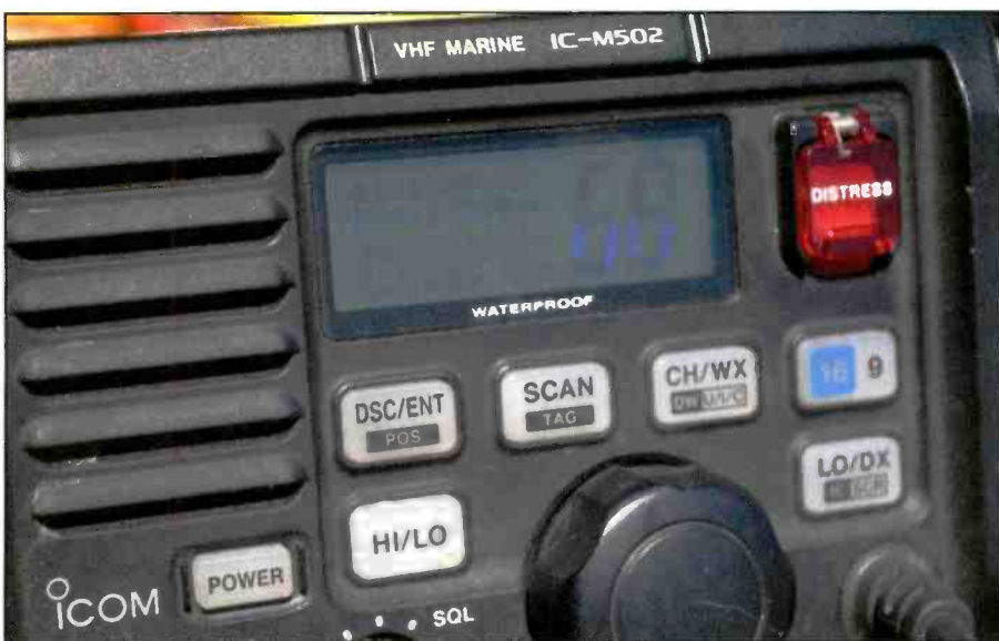
Photo E. You can spot a modern marine VHF radio with Digital Selective Calling by the red plastic cover that protects the distress “hot” button beneath it, as seen on the upper right of this marine radio. (Courtesy of WPC6NOA)
