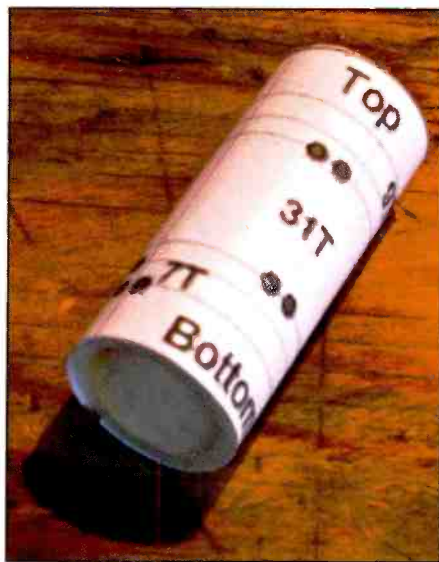
Photo F. Once the template is taped into place, it's a simple matter of drilling 1/16 th -inch diameter holes at the 12 places indicated.
