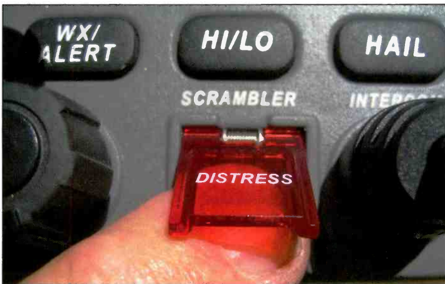
Photo F. A sailor in distress would lift the red DSC cover, push and hold the button for a few seconds, and the distress call would go out, digitally . The red plastic cover is spring-loaded to prevent an accidental activation. (Courtesy of WPC6NOA)
