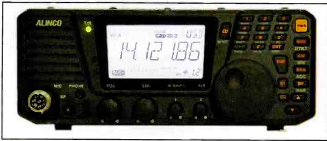
Photo E. For SWLing, the Alinco DX-SR8T has a dual-conversion superheterodyne receiver with a solid two-watts of audio and a receiver incremental tuning (RIT) range of +/- 1.2 kHz. (Internet screen grab < http://bit.ly/YTYaTX >)
