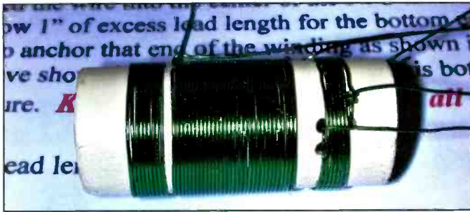
Photo I. Once completed, the Scout Regen's coil is a picture of green and white beauty. But is each winding's turn count correct?
