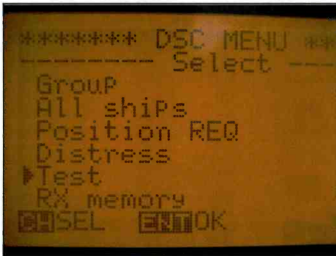
Photo G. Here is what the test screen looks like for contacting a local Coast Guard station to test DSC capabilities. (Courtesy of WPC6NOA)
