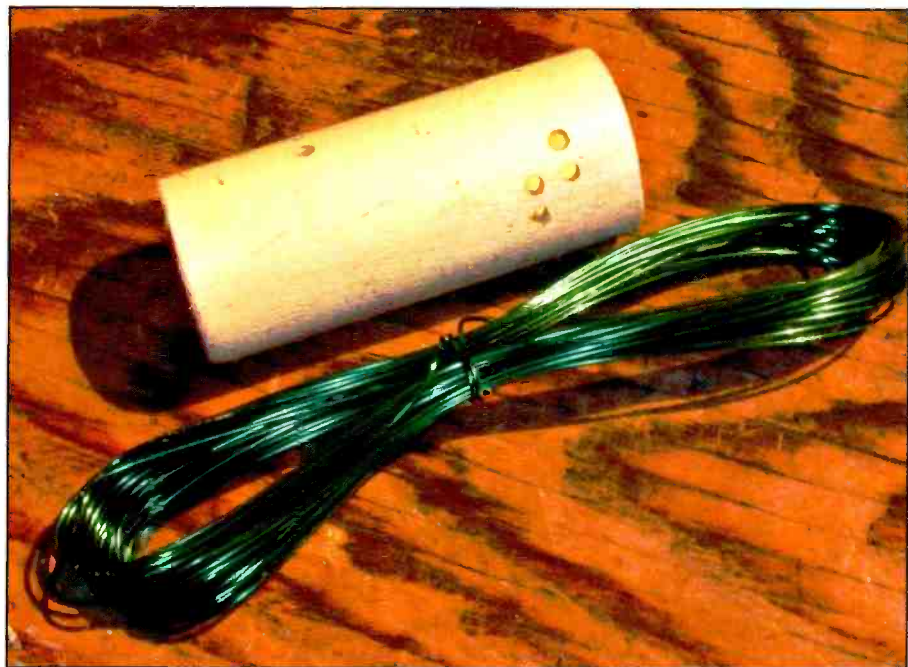
Photo G. Light sandpaper will remove any burrs after drilling, readying the PVC for three windings of No. 26 enameled wire.
