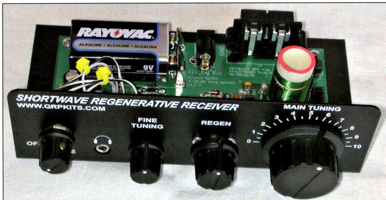
Photo A. The Hendricks QRP Kits Scout Regenerative Receiver is a handsome all solid-state kit designed for two coverage ranges: 3.3 to 5.1 MHz and 5.1 to 10+ MHz — perfect for shortwave AM and sideband monitoring, as well as “reading the mail” on some popular amateur bands. (Photography by KPC6PC)
