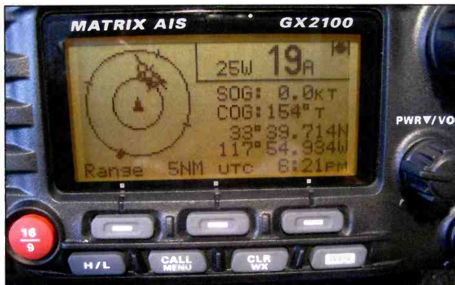
Photo K. This radio features an Automatic Identification System (AIS) that can allow the user to see other boats in the vicinity. (Courtesy of WPC6NOA)
